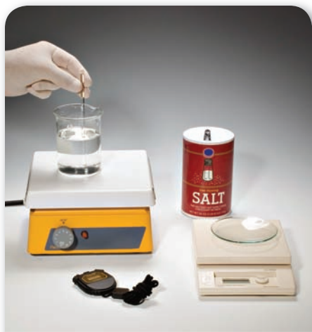
■ Figure 11 These materials can be used to determine the effect of temperature on the rate at which table salt dissolves.
